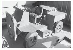
PSI 6,000 Lb. DBP Tug, 4-Cyl Chrysler Gas Engine, Auto Transmission, Calipers & Master Cylinders New Brake
