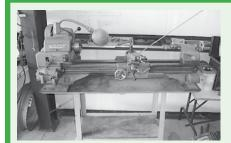
Craftsman Bench Top Lathe Quick Change, Variable Speed, 46" Bed, 36" Between Centers, 12" Swing w/Various Cutters, Steady Rest, Face Plate Tooling,
