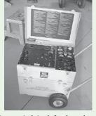
Howell Instrument Jetcal Analyzer/ Trimmer P/N BH112JB-53, 120V, 60-Cyl Complete w/All Probes, Etc.
