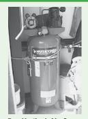
Husky Pro Vertical Air Compressor, 7-HP, 60-Gal Tank, 135 PSI Max Craftsman 15" Floor Mdl Drill Press, 12-Speed, 1-HP, 5/8 Chuck
