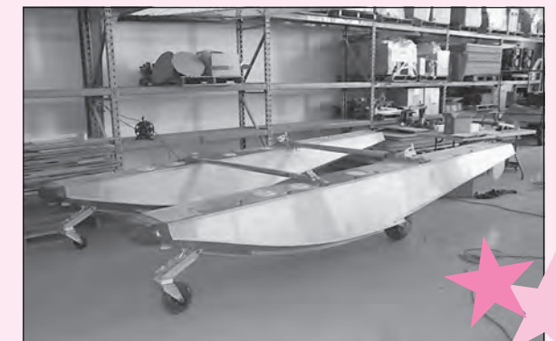
Set of Experimental Amphibious Floats for the Cubby
