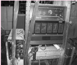
Miller Deltaweld 302 CV-DC Welding Power Source Miller XR Control Extended Reach Aluminum Wire Feed System w/ Miller XR-15A Air Cooled Wire Feed Gun
