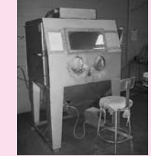
Trinco Bead Blast Cabinet, 48" x 36" w/ Filter & Reclaimer (5) Cylinder Working Tables w/Rotating Holding Fixture for Welding & Grinding
