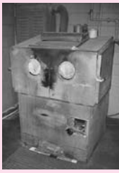
Zero Mdl D-100-F Bead Blast Cabinet, 42" W x 26" D x 23" T w/Filter & Reclaimer
