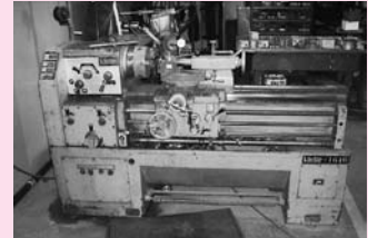
Victor 1640 High Speed Lathe, 15-3/4" Swing Over Bed, 40" Between Centers, 65-1800 RPM Spindle Speed
