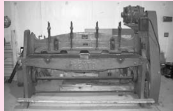
Pexto 6' Power Shear (Belt Driven), 16 Ga. Capacity
