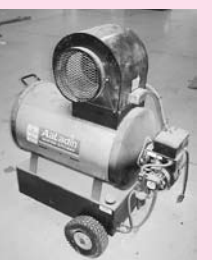
Aladdin Mdl 280 Portable Kerosene Space Heater 280,000 BTU w/Blower
