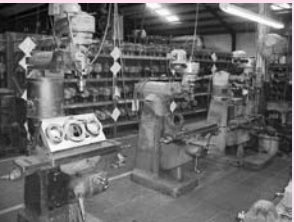
Bridgeport Vertical Milling Machine, 1 HP, 9" x 42" Table, Spindle Speed 80-2720 RPM w/7" Riser Block Bridgeport Vertical Milling Machine, 9" x 42" Power Feed Table, 1 HP, 80-2720 RPM Spindle Speed Bridgeport Vertical Milling Machine, 1 HP, 9" x 42" Power Feed Table, 80-2720 Spindle Speed, (2ea) 7" Riser Blocks
