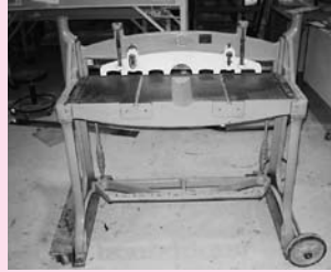
Pexto 36" Sheet Metal Shear, Mdl 137, 18 Ga. Capacity
