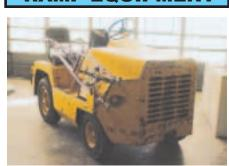
Clark Mdl. 2330237 Tug, 4,000 Lb. DBP, Auto Transmission, 6 Cvl. Ford Motor Yamaha Mdl. G/A Golf Cart. Gas Engine **B-4 Maintenance Stand**
