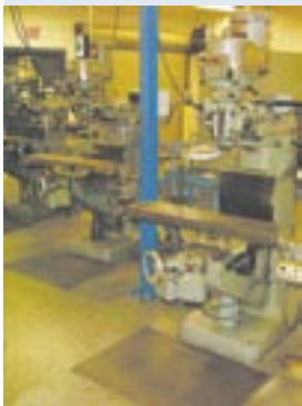
Bridge Port Series I Vertical Milling Machine 2H.P., XY Digital Read Out, 9" X 48" Three Slotted Table, Speed 80 RPM-4200 RPM w/ Rapid Traverse Bridge Port Series I Vertical Milling Machine 2H.P., XY Digital Read Out, 9" X 40" Three Slotted Table
