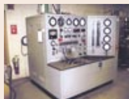
James A Staley Mdl D37885A Aircsearch APU Fuel Control Unit Test Stand w/10 HP Drive, Pressure Gauge Range from 0-1000 PSIG w/Up to 2600 PPH Fuel Flow
