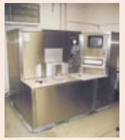
AAI/ACL Technologies Servo Valve Test Stand Mdl 9770-0117-1, S/N 03693-001 Skydrol Fluid, Flow & Press. 20 GPM @ 5000 PSI, Temp 120° F for 4-Way Flow Control & 3-Way Pressure Control Servo Valves
