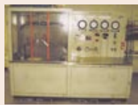
ACL Technologies Mdl 9770-0480 Universal Component Hyd. Test Stand S/N 2322-001, Flow & Pressure 50GPM @ 5000 PSIG, Temp 90-160° F, 125 HP D.C. Drive Motor, 1750-2500 RPM, Gear Box Speed 0-4000 RPM (low) 0-10,000 RPM (high) w/Sound Proof Enclosure
