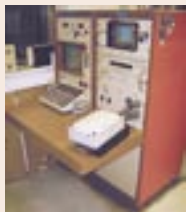
Avtron Mdl K738 CSD/Generator Test Stand, 300 HP Motor 1000 & 2170 RPM w/Max Spd of 2400 RPM, Gear Box 15,000 - 30,000 RPM Control Console P/N D20423 w/K731 Transient Recorder, Oscilloscope, K225 Modulation Meter, Computer Control w/619654 & A17638 Test Adapter, Load Bank etc. S/N 54
