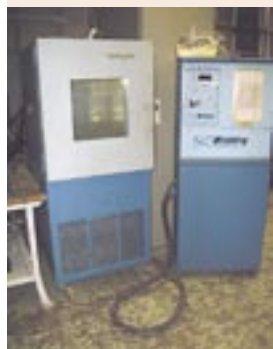
Tenney Mdl T.T.C Environmental Chamber, S/N 10949-11, Operating Range - 80° C To + 200° C, Inside 24" W x 27 3/4" H x 26" D
