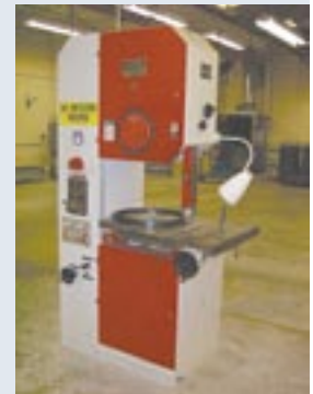
Dake Johnson Mdl. #V24 Vertical Band Saw w/23" Throat w/Blade Welder
