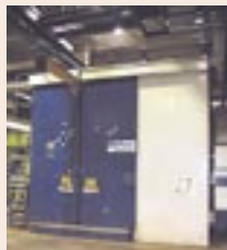
United Technologies Pratt & Whitney Engine ARMS Waterjet System. CNC Computer Controlled, Has Fanuc S-420 Robot, Kavel Robot Controller, 60" Diameter Rotary Table w/120" Part Capability. 55-150 Jet Edge Ultra High Pressure Pump, Quick Change Tooling Fixture Stand, Water Maze Water Cleaning System w/ AccuChiller, (2ea) Aerology Media Filter Modules Enclosure is 18' Wide x 35' Long
