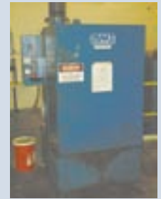
Mart Mdl Cyclone 2.2 Hot Water Rotary Parts Cleaner, 90 gal. Reservoir, Electric Heaters, 24" Rotary Table, S/N 6606, Mfg. 1996
