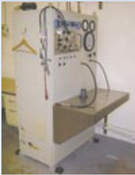
Monogram Sanitation Vacuum Toilet Pump Test Stand P/N 18000-001 Stainless Steel Clean Tank & Rinse Rack
