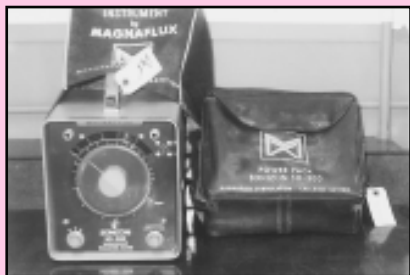
Magnaflux Sonizon SO-300 Ultrasonic Thickness Gauge w/Power Pack
