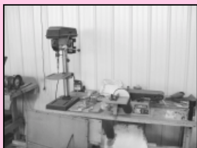
Variable Speed Bench Top Drill Press Delta 4" Belt and 6" Disc Sander
