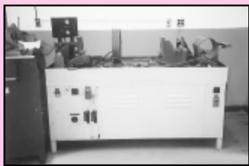
Magnaflux Machine, Spec. #50320-0, 6' Bed, DC, 5,000 Amp De-Mag Ring
