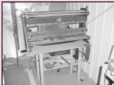
Enco Model 130-5-605 42" Press Brake and Sheet Metal Roller
