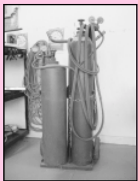
Oxygen Acetylene Torch Set w/ Cart and Bottles
